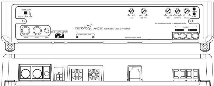
**GND**, +12V, **REM**: Please see previous page. These connections are the same as for the A150.1D. You MUST install a fuse holder with a 60A fuse within 18" (45cm) of the battery's + terminal.
