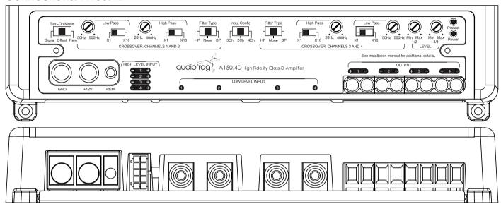
**GND:** Connect to the metal part of the vehicle's body. Scrape away paint to ensure a low resistance connection. Do not tin the wire with solder.
