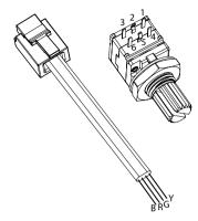
Connect the phone cord's black, red, green and yellow wires to the potentiometer according to the diagram below. Pins 2, 3, 5 and 6 must be connected together and to the black and green wires. Pin 1 must be connected to the yellow wire and pin 4 must be connected to the red wire. You can connect several amplifiers to one potentiometer in this manner.
